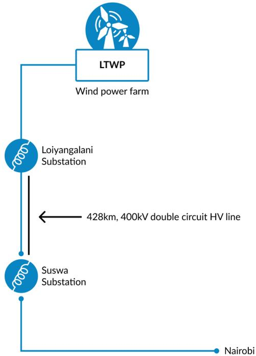
Figure 3.2: Schematic of the Lake Turkana Wind Project Transmission Line
